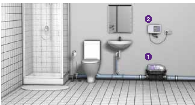
1 Backwater pumping station 2 Control unit
